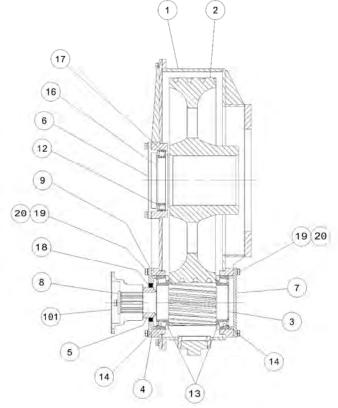
Figure 8: OPI-600 Gear Box Assembly Section A-A
