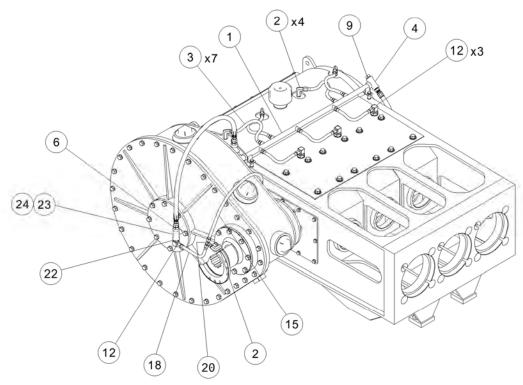
Figure 9: OPI-600 Lube Assembly, Drive Side View
